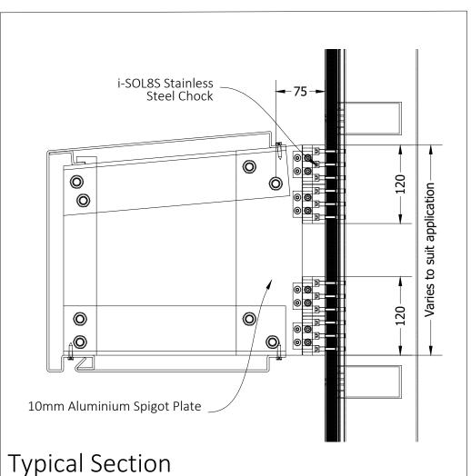
i-SOL8S curtain wall bracket adaptors are modular build components.
